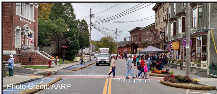
Figure 19 - Straw Wattle Bulb-out
